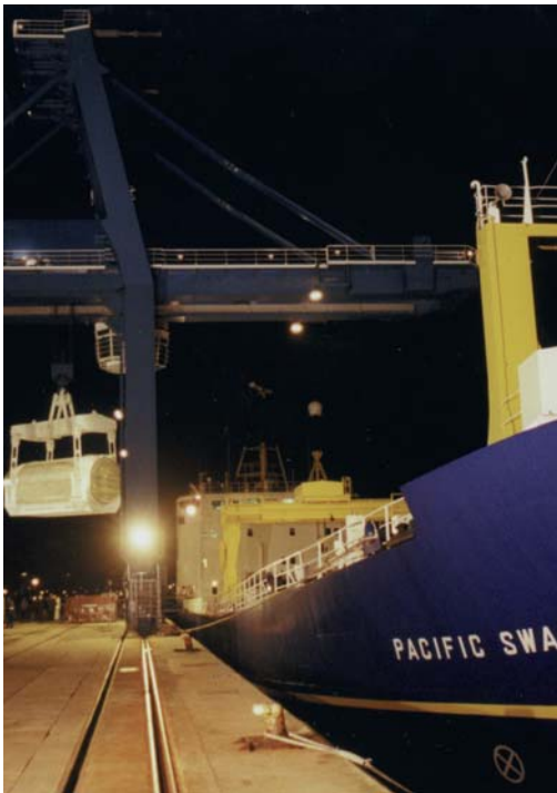
Loading a cask of vitrified residue onto a PNTL ship
