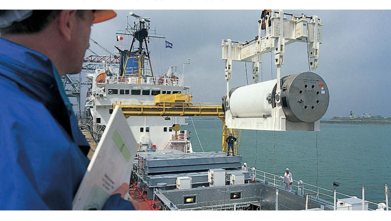
Its ships are dedicated to the transportation of nuclear material that is classified by the International Maritime Organization (IMO) of the United Nations at its highest level of "Class INF 3". The "INF Code" regulates shipments by sea of used (spent) fuel, plutonium and highly radioactive waste.
